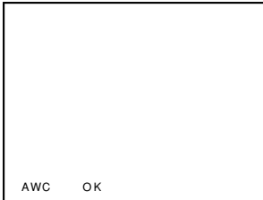
Indication when operation is completed normally.
